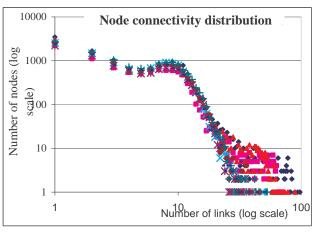
**Figure 5:** Connectivity distribution during November 2000. Each series of points represents one Gnutella network topology we discovered at different times during that month. Note the log scale on both axes. Gnutella nodes organized themselves into a power-law network.
