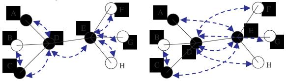
**Figure 7:** Gnutella's virtual network topology (blue, dotted arrows) mapping on the underlying network infrastructure (black). Left picture: perfect mapping. Right picture: inefficient mapping; link D-E needs to support six times higher traffic.
